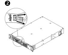
• Press and hold the black switch (see location designation below) to the right, while removing the power processing module.
